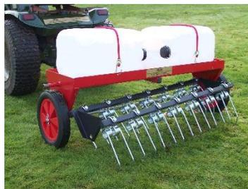
The tines are not designed to penetrate the soil, they tease through the mat of grass to pull out dead thatch.
